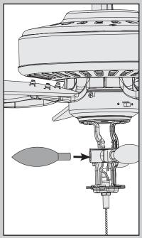
Install a light bulb in each socket.
