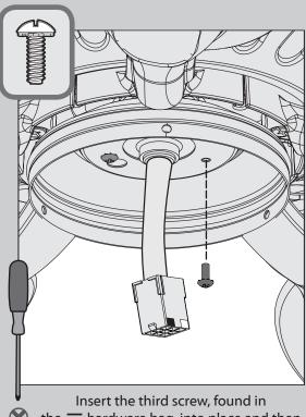
the hardware bag, into place and then tighten all three (3) screws.
