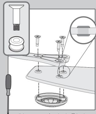
Install the grommets, found in the hardware bag, in the blades by hand. Place each blade between a blade iron and medallion. Install three blade screws, found in the hardware bag, to attach the medallion to the blade iron. Repeat for all blades.
