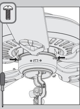
Install the third switch housing screw.
